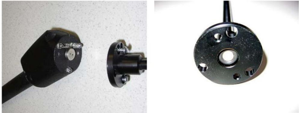
Fig. 18: Sinter filter in the sniffer handle
