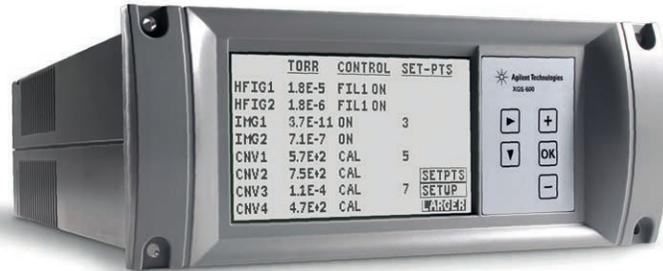
The XGS-600 Vacuum Gauge Controller provides unprecedented capacity, performance and flexibility in a cost effective, standard half-rack package. A single controller can simultaneously operate up to four hot filament (or four cold cathode) gauges and four convection gauges, up to five cold cathode gauges, or up to twelve convection gauges. Expansion or re-configuration in the field is easy to do. Serial communications (RS-232 or RS-485), eight set points, and universal voltage compatibility are
